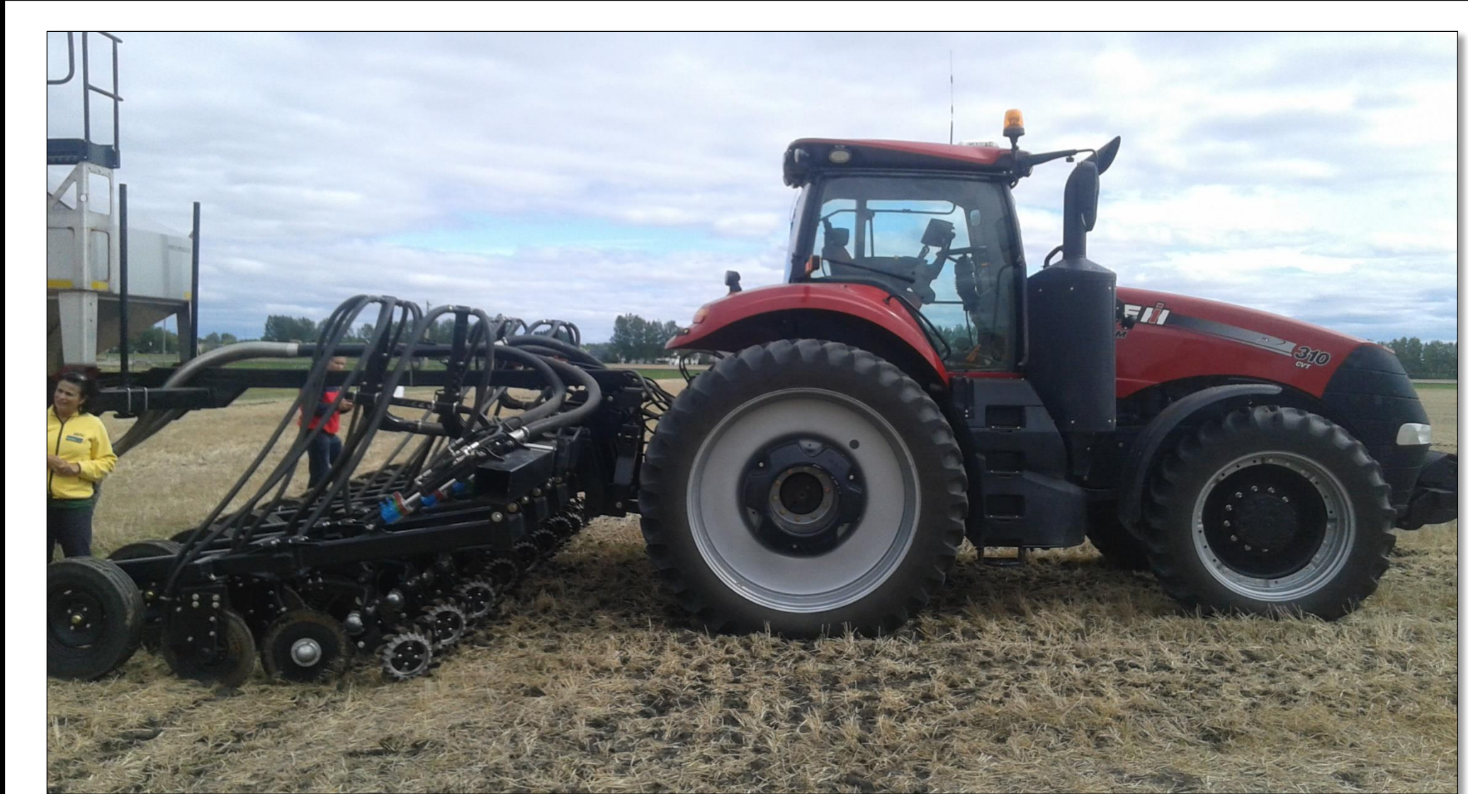
Figure 5. Prototype cover crop interseeder equipped for a simultaneous in-furrow side-dress N application.
