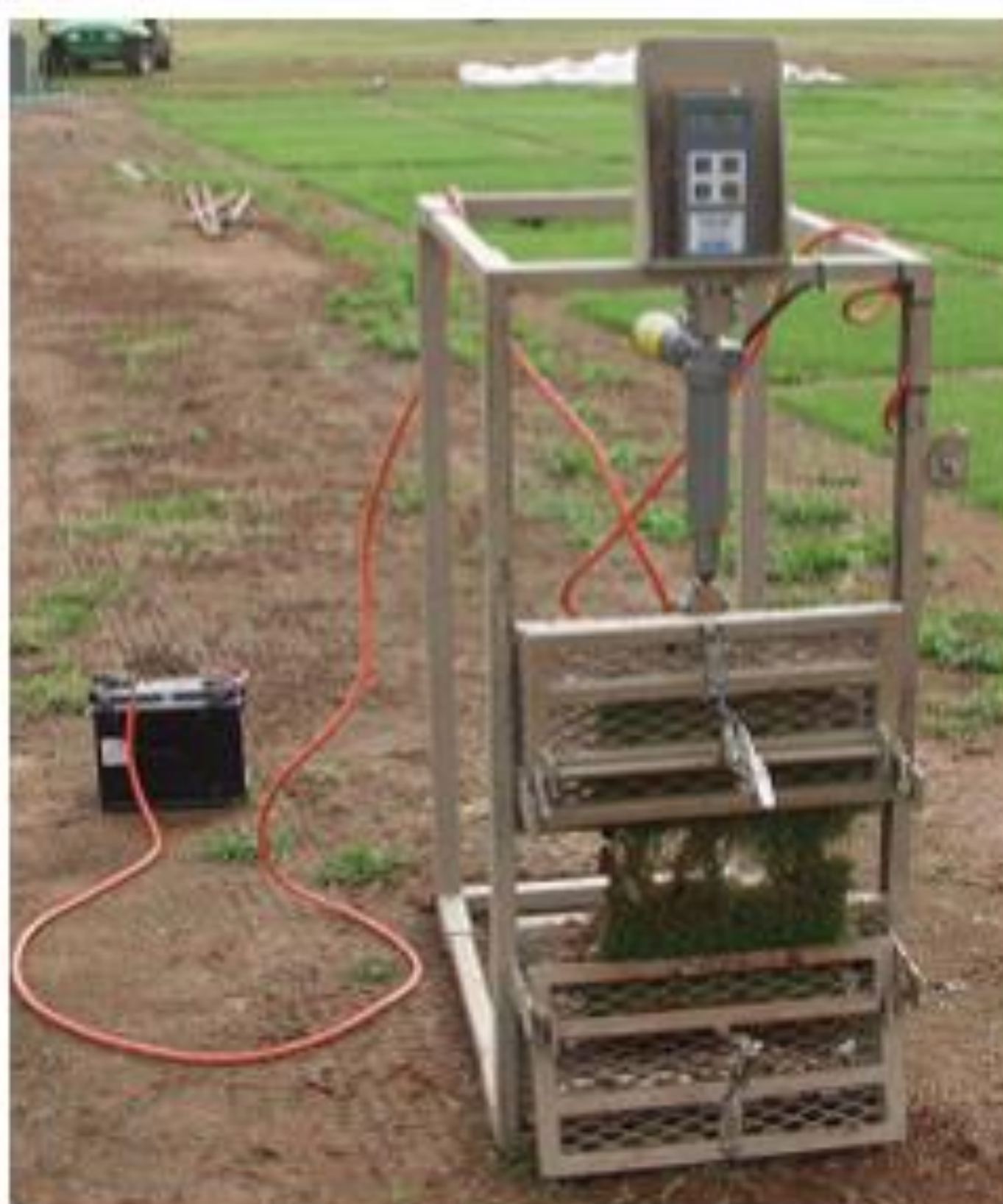
Figure 3: Sod tensile strength measurement device with force transducer/recorder system.
