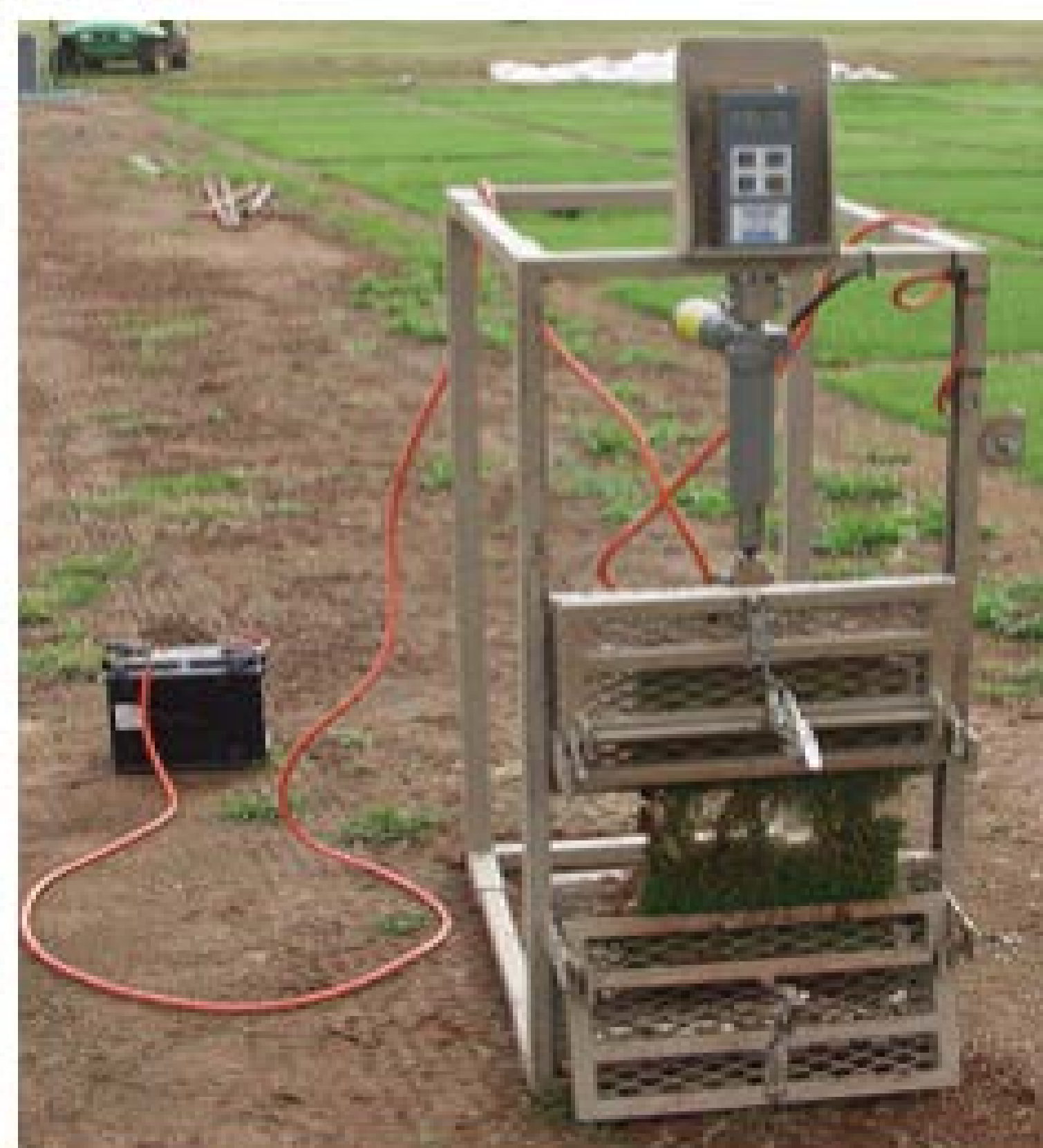
Figure 2: Sod tensile strength (STS) was measured under field conditions using a portable tensile strength machine.
