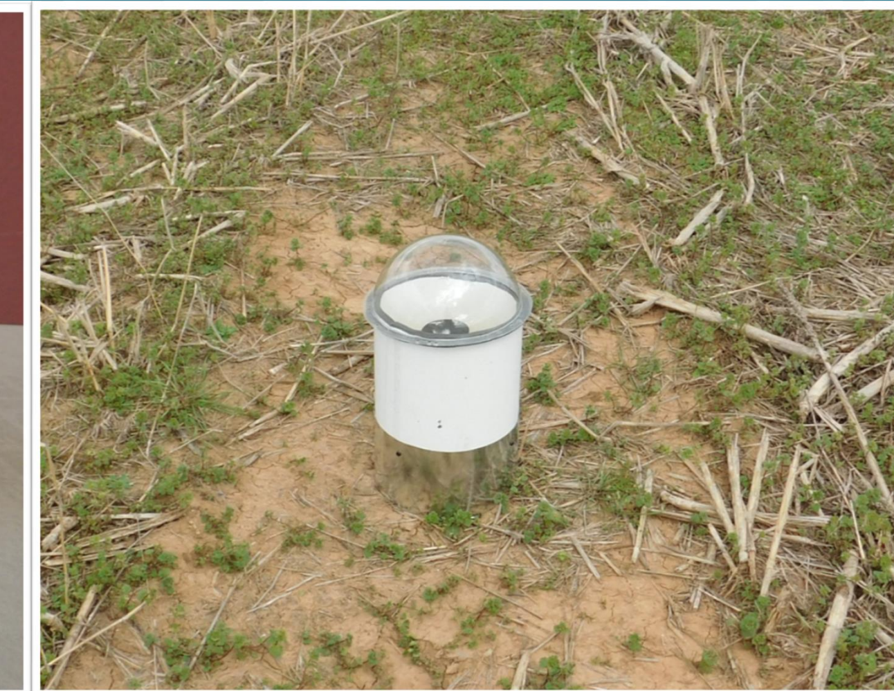
Figure 2. Home-made setup for CO 2 measurement
