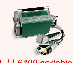
Fig. 2. LI-6400 portable photosynthesis system
