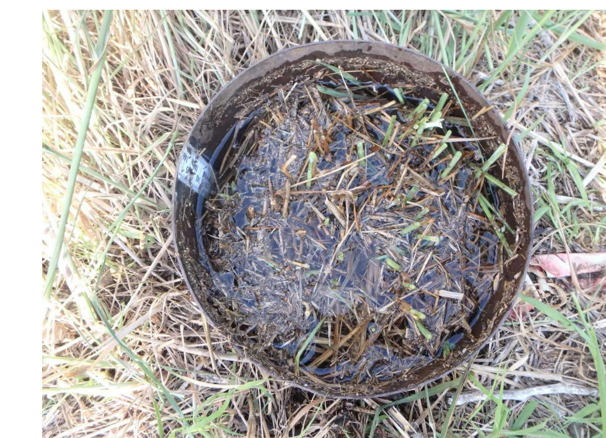
Fig. 4. Single ring infiltrometer method
