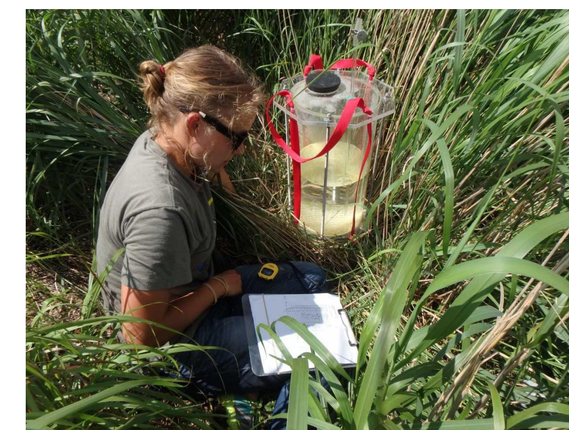
Fig. 5. Cornell infiltrometer method
