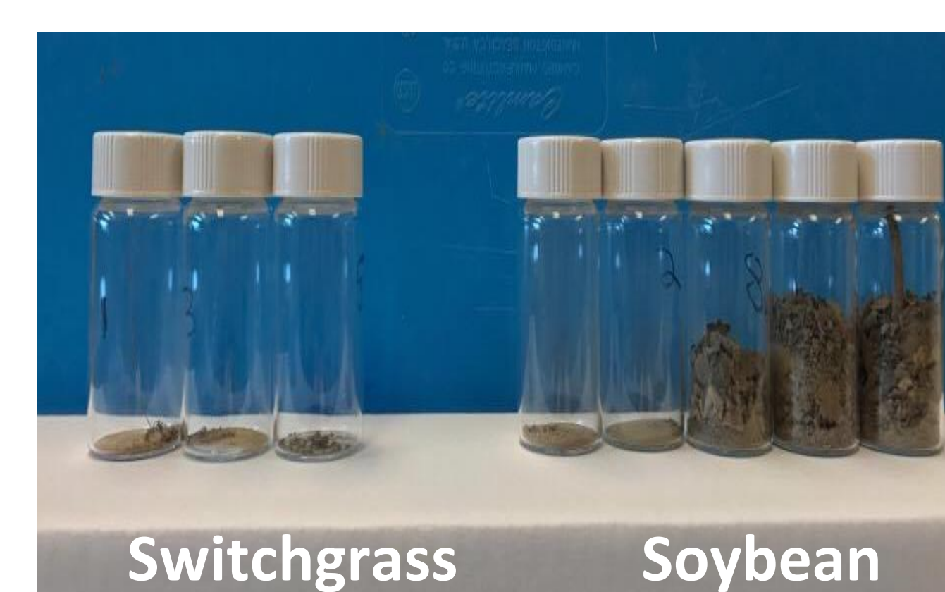
Fig. 9. Sediment in runoff collected with the Cornell infiltrometer
