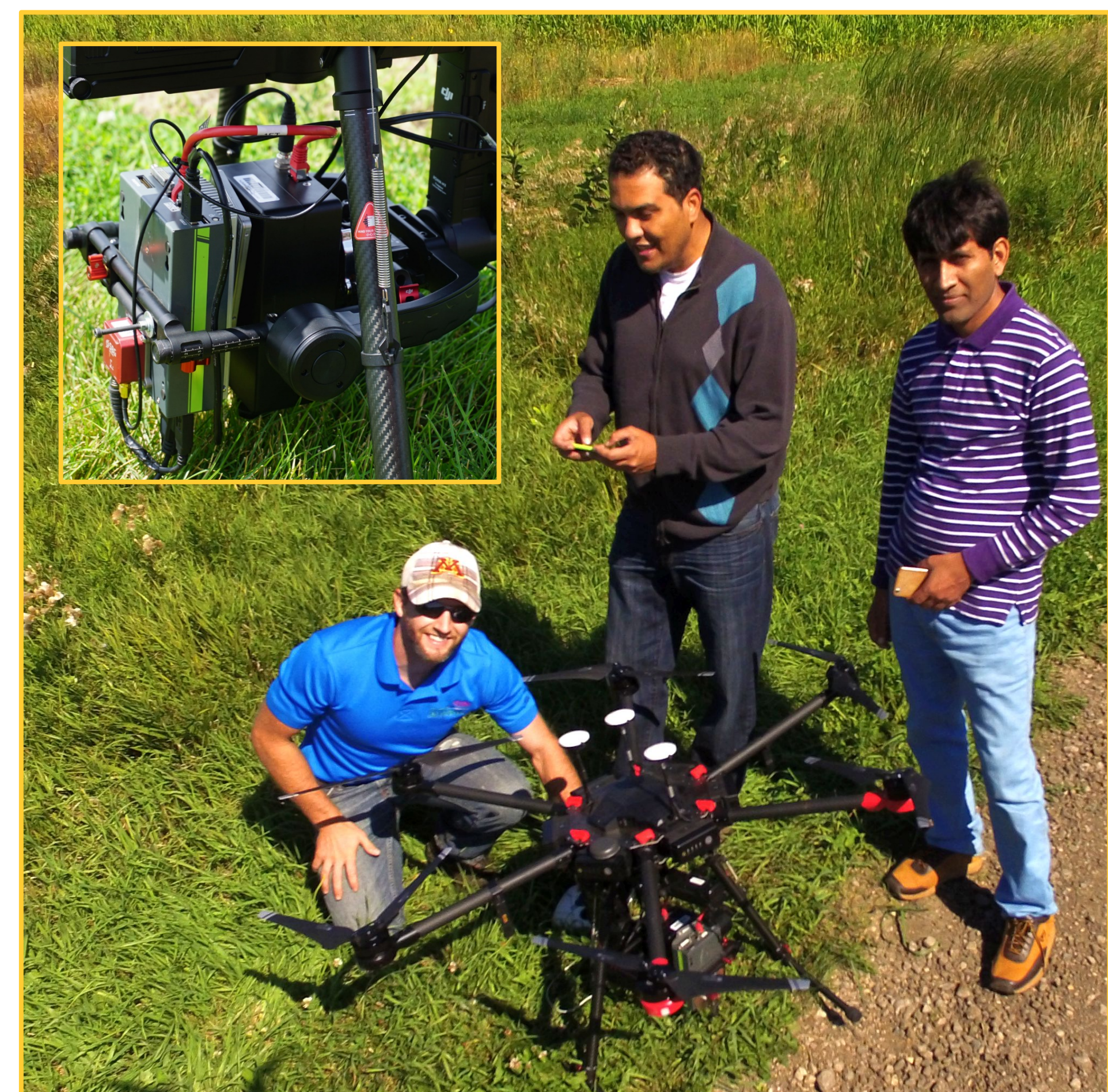
Figure 1: Muhammad Tahir (right), Aicam Laacouri (middle), and myself (left) preparing the hexacopter and gimbal-mounted hyperspectral camera (inset photo) for aerial image acquisition.
