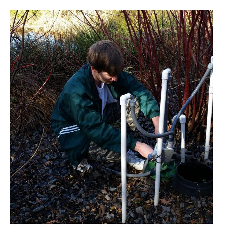
Taking a water sample from the lysimeter
