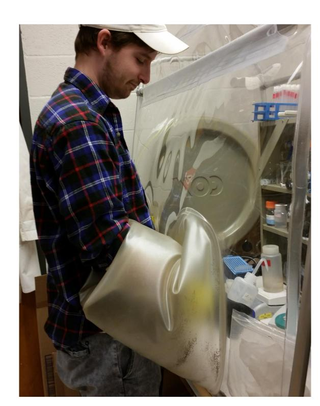
Preparing ferrozine-standard recipe in the glovebox in order to complex Fe<sup>2+</sup> in the field
