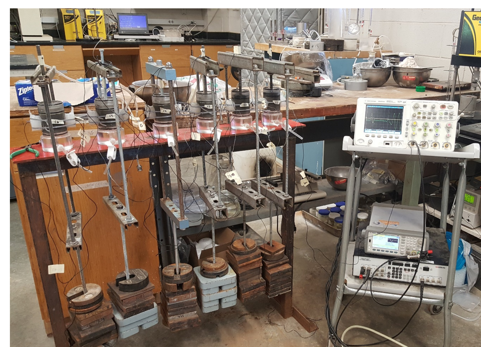
Above: Experimental set-up and oscilloscope used to measure shear wave velocity through treatment.
