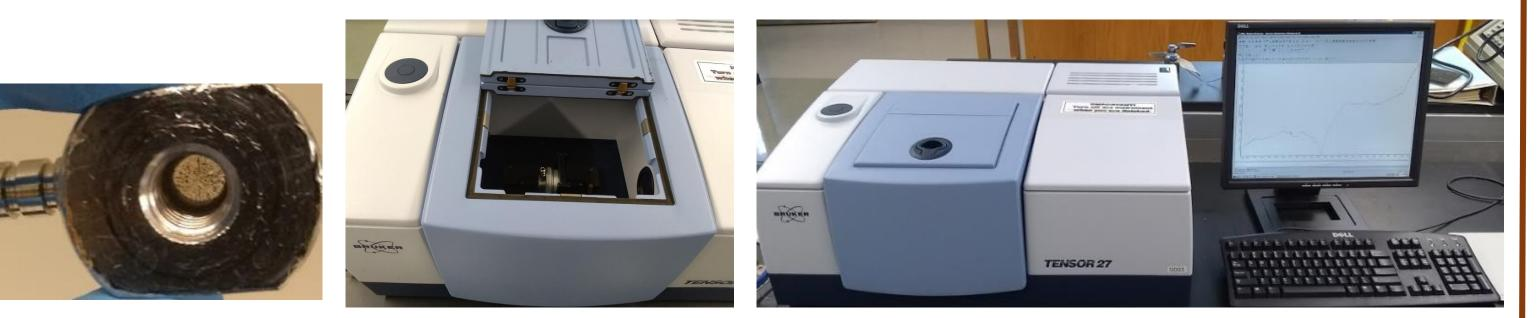
KBr pellet press Bruker Tensor 27 (above pictures) used for the second and third methods
