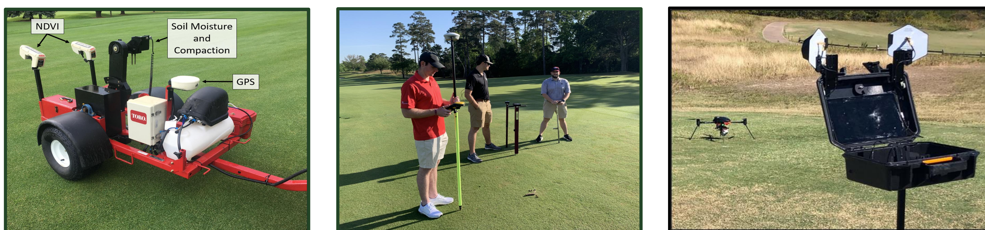
Figure 2. Image of the Precision Sense 6000 (left), GPS Trimble Geo7x (center), and Dragonfly Commander 2 with MicaSense Altum-PT (right)
