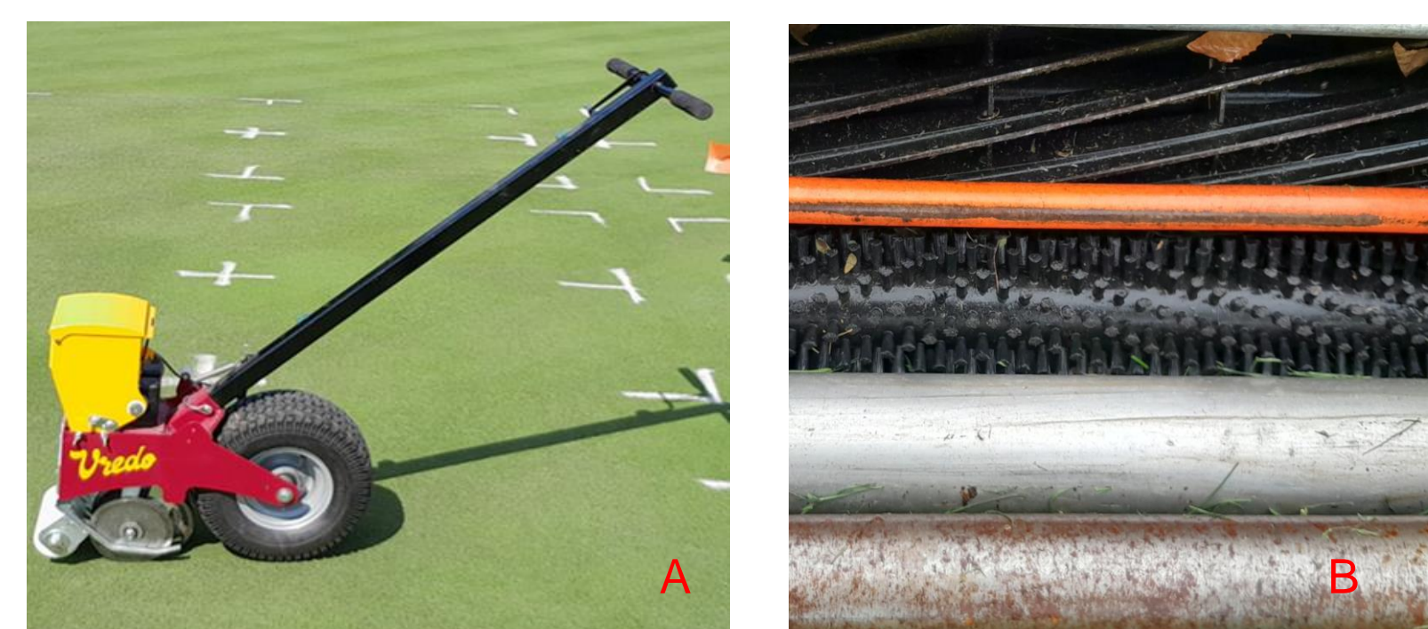
Figure 2. Vredo Turf Buddy Slit seeder (A), Brushing unit (B) attachment on walk mower.
