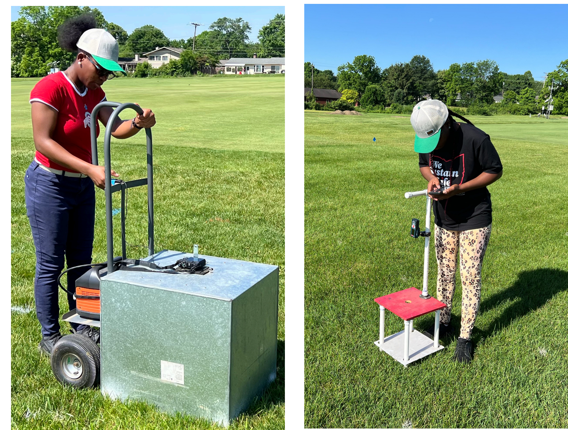
Figure 1. Dark green color index was quantified via images collected through a light box (left). Turfgrass height was assessed using a Turf Height Tester (right).
