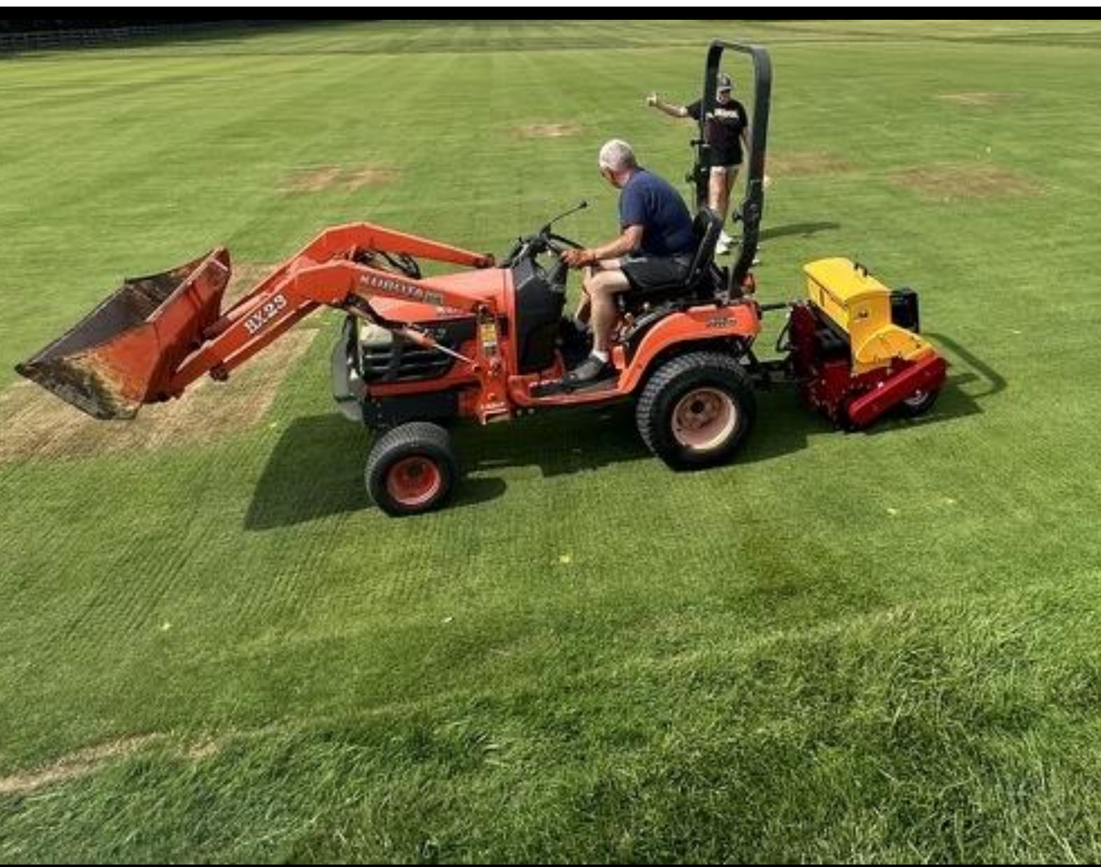
Vredo Turf-Fix 25" interseeding study plots at W.H. Daniel Turfgrass Research & Diagnostic Center, Purdue University
